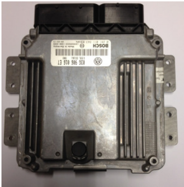
Large ECU: larger than adapter plate.
