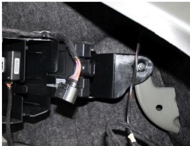
Disconnect the control unit for the sound generator.
